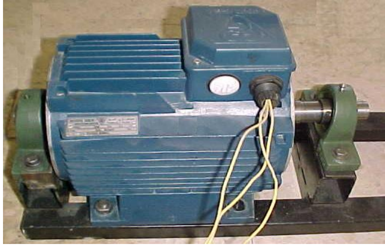
Fig. 5. Induction motor with moveable bearings.
